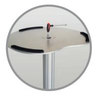
**WARNING** – large base plate is heavy (7.5kg). Position base plate over 8-way post and align 4 off fixing holes to threads of post (ensuring the countersunk holes are uppermost). Insert and tighten 4 off base plate screws to secure.
