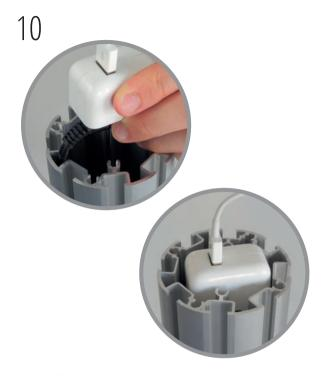
Position black mains cable into internal post channel, and carefully slide USB Power Adapter inside post so the USB head of charge/sync cable is below upper edge of post.
