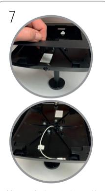
Lift fascia out of enclosure. Gently press cable (supplied with Apple iPad) into retaining moulding, allowing 10cm to remain "free" at charge/sync connector end.
