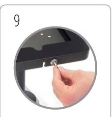
Unlock each iPad enclosure by inserting key into security lock and rotate 'QUARTER TURN ONLY' clockwise or counter-clockwise through 90 degrees, which releases the locking pin. Return key back to original position to remove.
