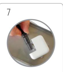
Plug one figure 8 head into a USB Power Adapter (supplied with Apple iPad) and position into retaining pins. Repeat for remaining power leads and adapters.
