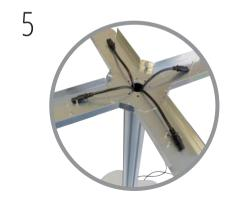
Feed figure 8 heads of power leads through central hole of bottom support plate and carefully place plate onto post. Align 4 holes to threads inside post at desired display angle.
