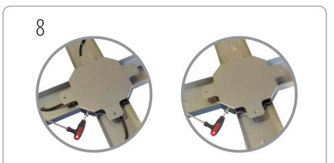
Carefully position and lower octagonal centre cover onto bottom support plate. Align two side holes of cover to any thread fixings of bottom support plate. Insert and tighten two hex socket screws to secure octagonal centre cover.
