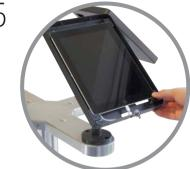
Plug charge/sync cable into one iPad and place inside enclosure, gently press all four corners of iPad down into mouldings to hold. Repeat for remaining iPads.
