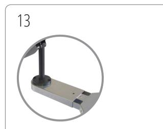
Carefully position and slide top support plate onto end of bottom support plate, ensuring the internal cables do not interfere with this assembly.
