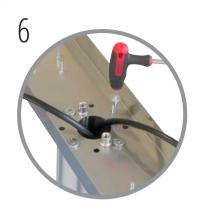
Insert and tighten 4 off base plate screws to secure.
