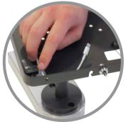
Lift fascia out of enclosures. Insert cables (supplied with Apple iPad) into both holders, allowing 10cm to remain "free" at charge/sync connector end by gently pressing into retaining moulding.
