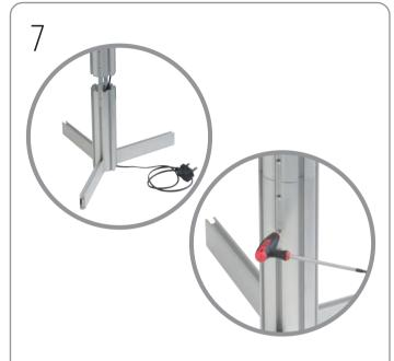
Connect the 1m and 265mm posts by locating connector bars into channels and sliding together. Tighten remaining grub screws to affix.
