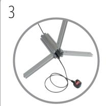
Feed figure-8 head of power lead through bottom of post and profiles assembly, leaving approximately 1m of cable at bottom.
