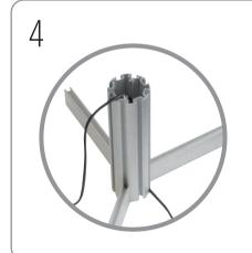
Stand post and profiles assembly upright ensuring lead is kept clear of foot screws.
