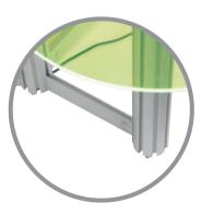
Starting with the smallest Podium table, position and slot clamp of one 220mm profile into post channel. Close T-Loc lever to attach. Repeat process for medium and large Podium tables.
