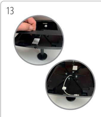
Lift fascia out of enclosure. Insert cable (supplied with Apple iPad) allowing 10cm to remain "free" at charge/sync connector end by gently pressing into retaining moulding.
