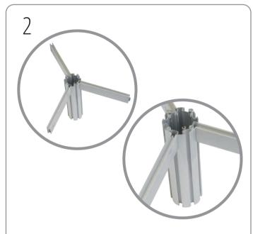
Take 265mm post and slot clamp of three 220mm profiles into desired channels for display. Ensure bottom of profiles are flush with bottom of post and close T-Loc lever to secure in position.
