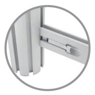
Position remaining 220mm profiles between posts near underside of Podium tops. Insert clamps into channels and secure by closing T-Loc lever.
