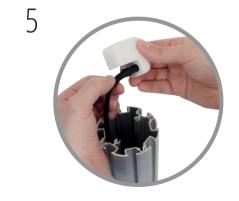
Plug figure-8 head into USB Power Adapter (supplied with Apple iPad).
