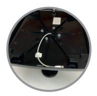
Plug charge/sync cable into iPad and place inside enclosure, gently press all four corners of iPad down into mouldings to hold.
