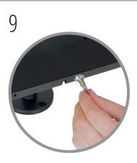
Unlock the iPad enclosure by inserting key into security lock and rotate 'QUARTER TURN ONLY' clockwise or counter-clockwise through 90 degrees which releases the locking pin. Return key back to original position to remove.
