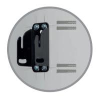
For brick/concrete walls, use 8mm masonry bit to drill 4x holes. Insert 4x rawl plugs and secure back plate of mount using screws and washers supplied.
