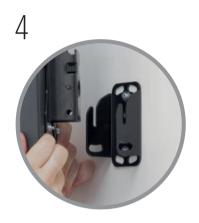
Position assembled iPad enclosure and VESA plate over wall mount and lower until both locating pins rest in bracket channels.
