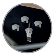
Feed USB end of charge/sync cable through middle of enclosure, below pin, so it protrudes from underside of counter/table top.
