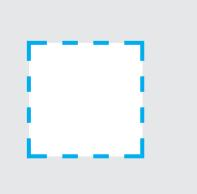
**Hinged Fold Area:** Blue lines indicate hinged area where body panel is folded and must have a gap in the graphic of 2/3mm.
