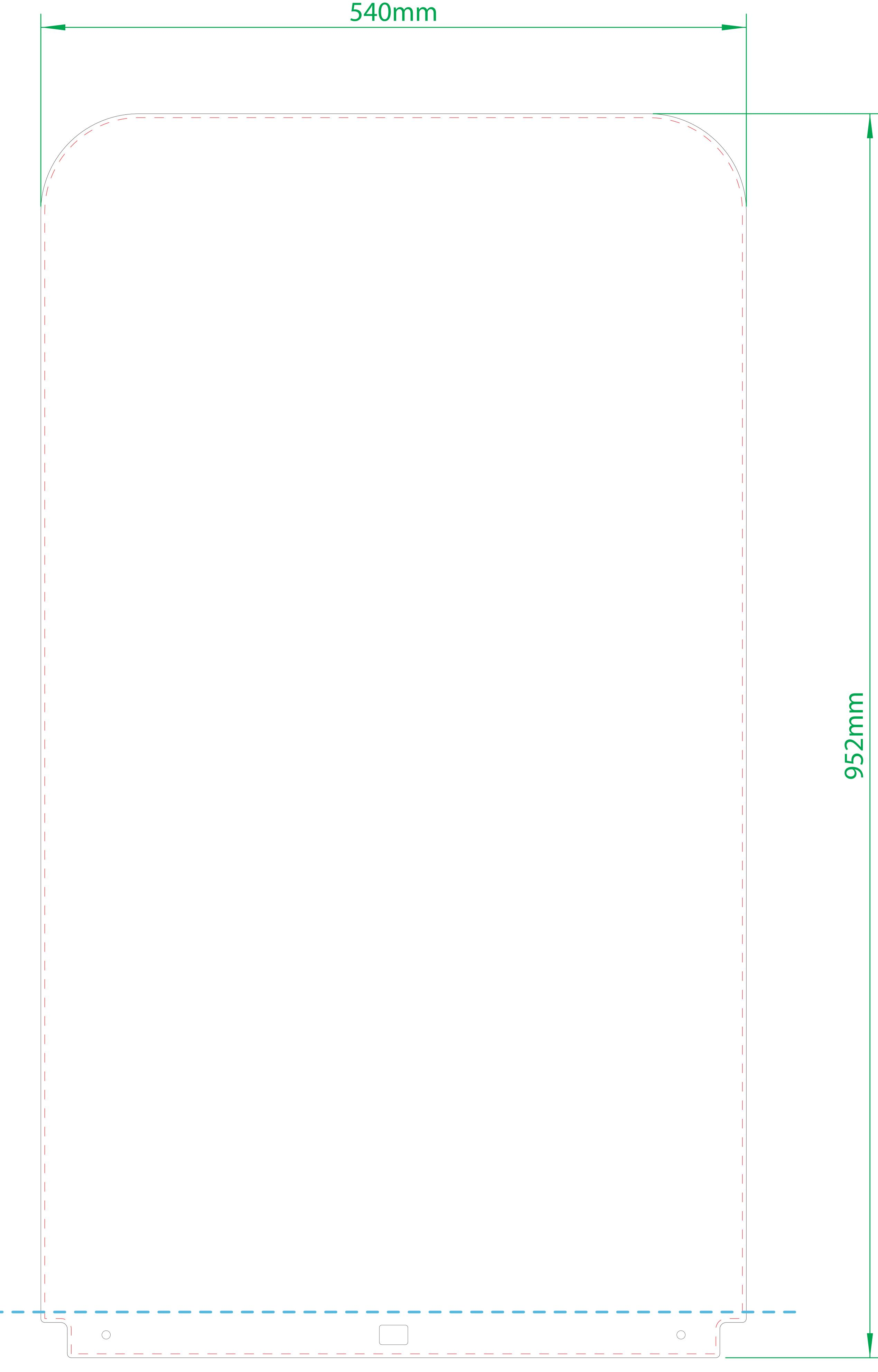
PLEASE NOTE: THIS AREA UNDERNEATH THE BLUE DASHED LINE IS NOT VISIBLE WHEN PANEL SLOTS INTO BASE.
